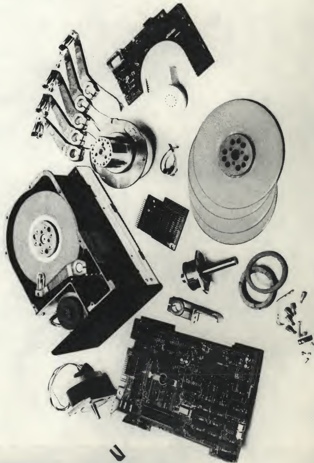
Component parts of RO200 series disk drive
